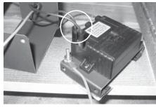
12) Install the supplied battery into the DC Sparker Box by opening the battery compartment.
